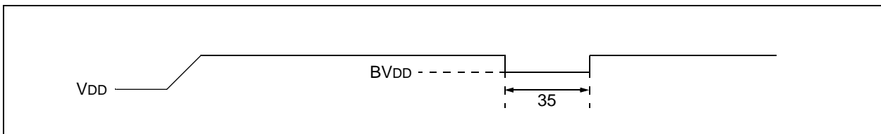
FIGURE 16-7: BROWN-OUT RESET TIMING
